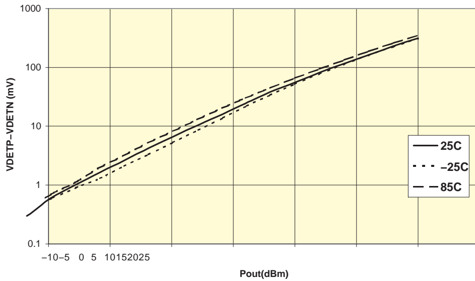
Figure 2. B Band Detector Output
