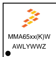
Figure 3. Device Orientation Diagram
