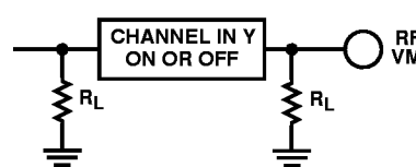
FIGURE 22. CROSSTALK BETWEEN DUALS OR TRIPLETS (CD4052B, CD4053B)
