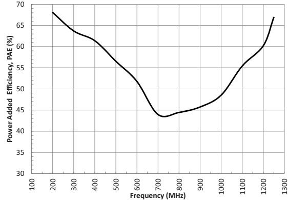
PAE versus Frequency, P_{OUT} = 39.5dBm (CW, V_D = 28V, I_{DQ} = 88mA )
