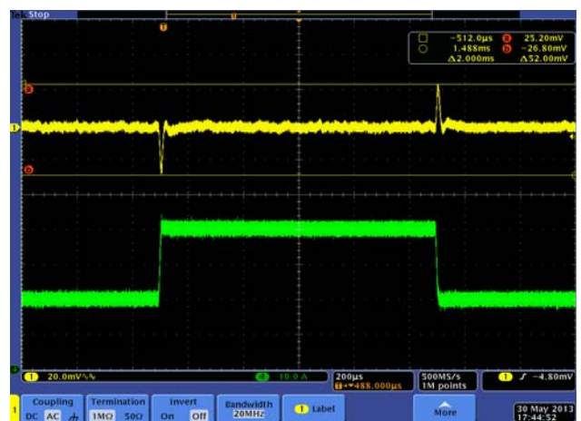
FIGURE 14. STEP RESPONSE, 20A TO 40A @ 5A/µs, ASCR = 400 TOTAL DEVIATION WINDOW 50mV = 5%
