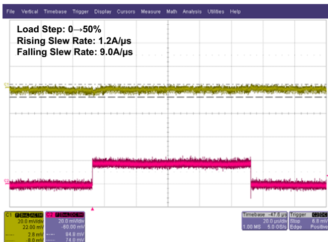
Figure 32. Load Transient Waveform
