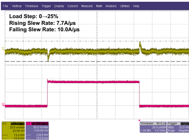
Figure 35. Load Transient Waveform
