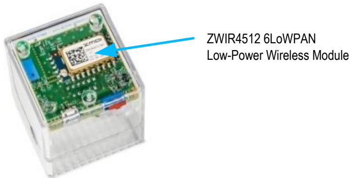
Figure 2. Bottom View of Sensor Cube
