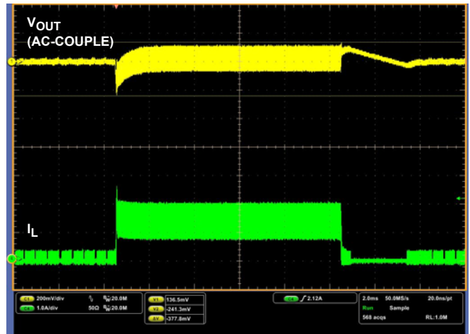
FIGURE 11. LOAD TRANSIENT RESPONSE 0A->1A, VIN = 36V
