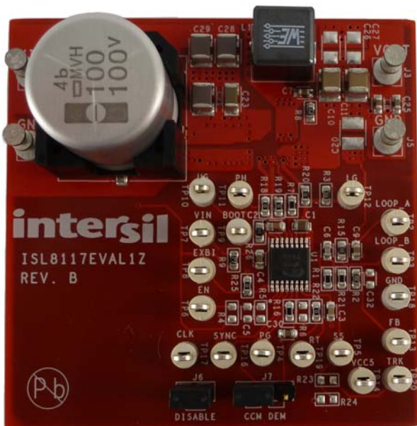
FIGURE 1. ISL8117EVAL1Z TOP SIDE
