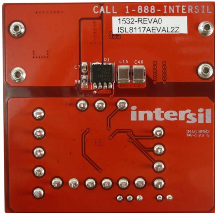
FIGURE 5. ISL8117AEVAL2Z BOTTOM SIDE
