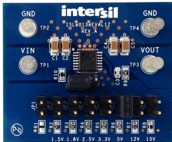
FIGURE 1. ISL80138EVAL1Z EVALUATION BOARD
