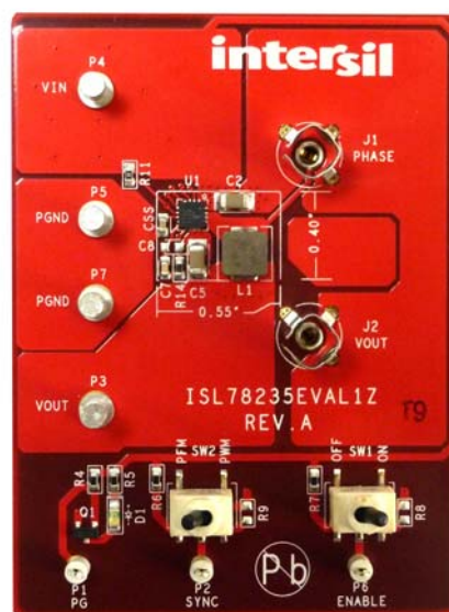
FIGURE 1. ISL78235EVAL1Z EVALUATION BOARD PHOTO
