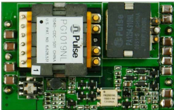
FIGURE 1. TOP VIEW OF ISL6726EVAL1Z (ACTUAL SIZE: 40x60x16mm)
