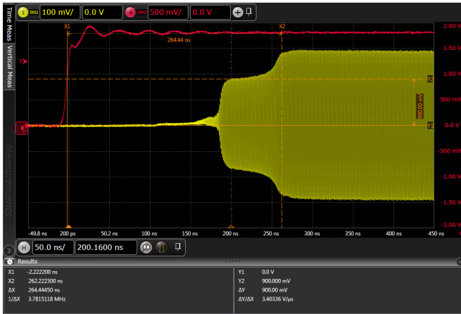
Figure 16. Switching Time Isolation to Insertion loss
