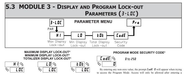
These displays can be programmed for LOC or rEd. When programmed for LOC, the display will not be shown when the **DSP** key is pressed regardless of Program Lock-out status. It is suggested to lock-out the display if it is not needed. The associated function will continue to operate even if its display is locked-out.
