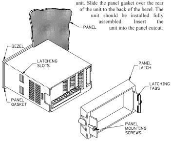
While holding the unit in place, push the panel latch over the rear of the unit so that the tabs of the panel latch engage in the slots on the case. The panel latch should be engaged in the farthest forward slot possible. To achieve a proper seal, tighten the latch screws evenly until the unit is snug in the panel (Torque to approximately 7 in-lbs [79N-cm]). Do not over-tighten the screws.
