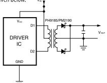
For a fixed 50% duty cycle mode of operation, the output voltage is simply determined by the input voltage and turns ratio. So, with the available turns ratios, a variety of output voltages can be selected.
