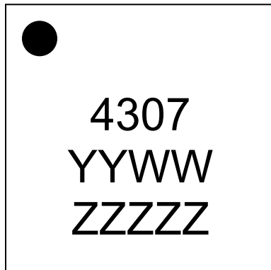
Figure 21. Top Marking Specifications
