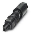
Photovoltaic connector, Range of articles: PV-CF-S, Connector, housing material: PPE, color: black, number of positions: 0, min. conductor cross section: 6 mm<sup>2</sup>, max. conductor cross section: 16 mm<sup>2</sup>, rated current: 40 A, Connection method: Spring-cage, Type of contact: Socket
