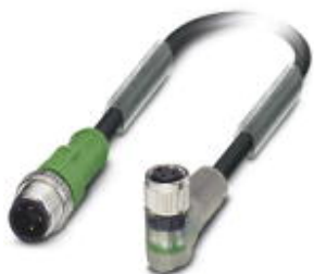
Sensor/actuator cable, 3-position, PUR halogen-free, black-gray RAL 7021, Plug straight M12, coding: A, on Socket angled M8, with 2 LEDs, cable length: 5 m
