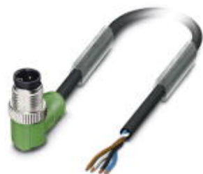
Sensor/actuator cable, 4-position, Variable cable type, Plug angled M12, coding: A, on free cable end, cable length: Free input (0.2 ... 40.0 m)
