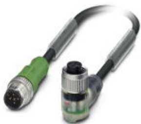
Sensor/actuator cable, 5-position, PUR halogen-free, black-gray RAL 7021, Plug straight M12, coding: A, on Socket angled M12, coding: A, with 3 LEDs, cable length: 0.6 m
