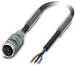
Sensor/actuator cable, 3-position, PUR halogen-free, black-gray RAL 7021, free cable end, on Socket straight M12, coding: A, with 2 LEDs, cable length: 3 m
