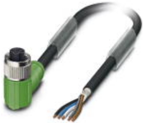
Sensor/actuator cable, 5-position, PUR halogen-free, black-gray RAL 7021, shielded, free cable end, on Socket angled M12, coding: A, cable length: 5 m
