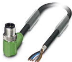
Sensor/actuator cable, 5-position, PUR halogen-free, black-gray RAL 7021, shielded, Plug angled M12, coding: A, on free cable end, cable length: 5 m
