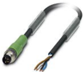
Sensor/actuator cable, 4-position, PUR halogen-free, black-gray RAL 7021, Plug straight M8, on free cable end, cable length: 3 m
