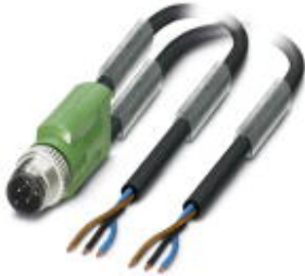
Sensor/actuator cable, 3-position, PUR halogen-free, black-gray RAL 7021, unshielded, Plug straight M12, coding: A, on free cable end and free cable end, cable length: 3 m
