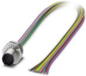
Sensor/actuator flush-type plug, 12-pos., M12 SPEEDCON, front/screw mounting with M16 thread, with 0.5 m PVC litz wire, 12 x 0.14 mm 2
