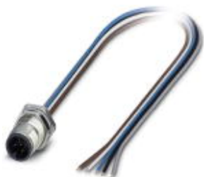
Sensor/actuator flush-type plug, 5-pos., M12 SPEEDCON, A-coded, rear/screw mounting with M12 thread, with 0.5 m TPE litz wire, 5 x 0.34 mm 2
