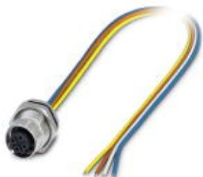
Bus system flush-type socket, PROFINET, 4-pos., M12 SPEEDCON, D-coded, front/screw mounting with Pg9 thread, with 0.5 m TPE litz wire, 4 x 0.34 mm 2
