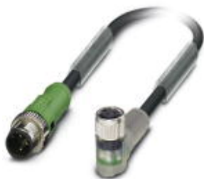
Sensor/actuator cable, 3-position, Variable cable type, Plug straight M12 SPEEDCON, coding: A, on Socket angled M8, with 2 LEDs, cable length: Free input (0.2 ... 40.0 m)
