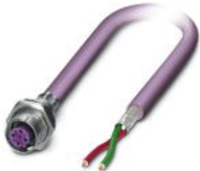
Bus system flush-type socket, PROFIBUS, 2-pos., M12, shielded, B-coded, rear/screw mounting with M16 thread, with 5 m bus cable, 2 x 0.25 mm 2
