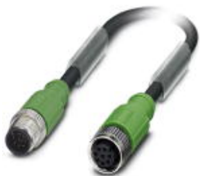
Sensor/actuator cable, 8-position, PUR halogen-free, black-gray RAL 7021, shielded, Plug straight M12, coding: A, on Socket straight M12, coding: A, cable length: 3 m
