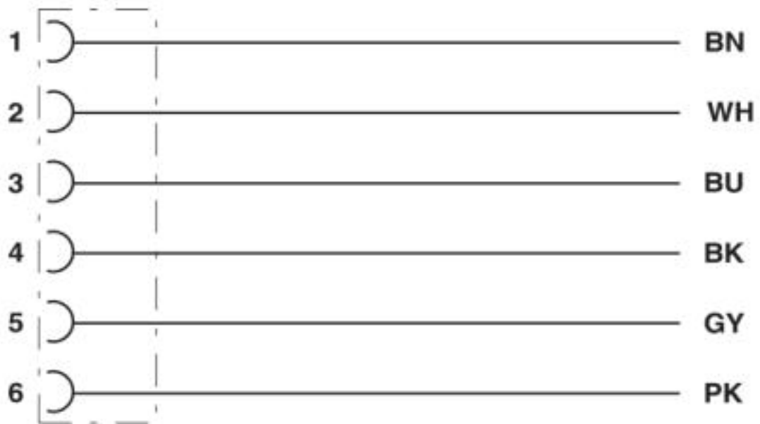
Contact assignment of M8 socket
