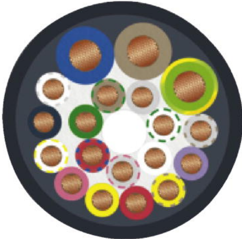
Cable cross section
