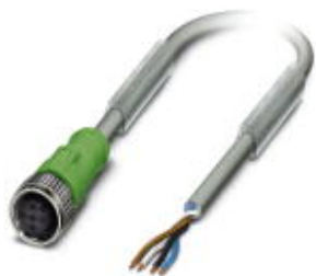
Sensor/actuator cable, 4-position, PUR halogen-free, resistant to welding sparks, highly flexible, gray RAL 7001, free cable end, on Socket straight M12, coding: A, cable length: 1.5 m, for robots and drag chains
