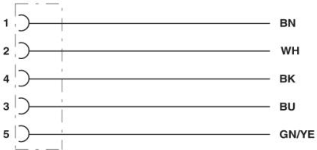
Contact assignment of the M12 sockets
