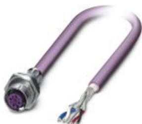
Bus system flush-type socket, DeviceNet/CANopen, 5-pos., M12, shielded, A-coded, Speedcon, rear/screw mounting with Pg9 thread, with 0.5 m bus cable, 2 x 0.2 mm²; 2 x 0.32 mm²
