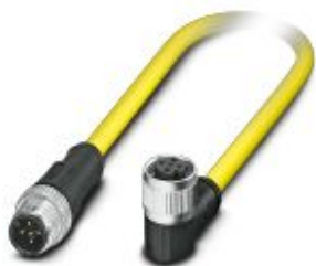
Sensor/actuator cable, 5-position, PVC, yellow, Plug straight M12 SPEEDCON, coding: A, on Socket angled M12 SPEEDCON, coding: A, cable length: 5 m
