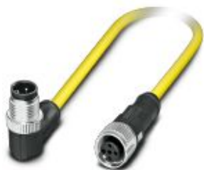
Sensor/actuator cable, 3-position, PVC, yellow, Plug angled M12 SPEEDCON, coding: A, on Socket straight M12 SPEEDCON, coding: A, cable length: 5 m
