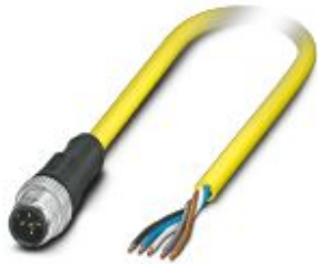
Sensor/actuator cable, 5-position, PVC, yellow, Plug straight M12 SPEEDCON, coding: A, on free cable end, cable length: 5 m
