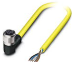
Sensor/actuator cable, 5-position, PVC, yellow, free cable end, on Socket angled M12 SPEEDCON, coding: A, cable length: 10 m
