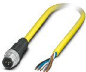
Sensor/actuator cable, 5-position, PVC, yellow, Plug straight M12 SPEEDCON, coding: A, on free cable end, cable length: 10 m
