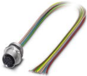
Flush-type connector, Universal, 8-position, Socket, straight, M12-SPEEDCON, A-coded, Front mounting, M16 x 1.5, Individual wires, cable length: 1.2 m, 0.25 mm 2 , TPE litz wire
