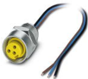
Flush-type connector, 3-position, Socket, straight, 7/8"-16UNF, on free cable end, Front mounting, with 1/2 inch-14 NPT mounting thread, Individual wires, cable length: 1 m, 0.75 mm 2 , PVC litz wire
