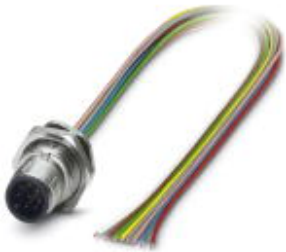
Sensor/actuator flush-type plug, 8-pos., M12 SPEEDCON, rear/screw mounting with M16 thread, with 0.5 m TPE litz wire, 8 x 0.25 mm 2
