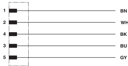
Contact assignment of the M12 plug
