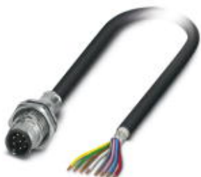
Flush-type plug, shielded, 8-pos., M12, A-coded, rear/screw mounting with M16 thread, with 1 m cable, 8 x 0.25 mm 2
