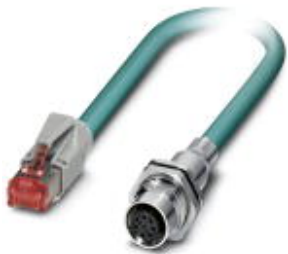
Network cable, number of positions: 8, 1 Gbps, CAT5, cable outlet: straight
