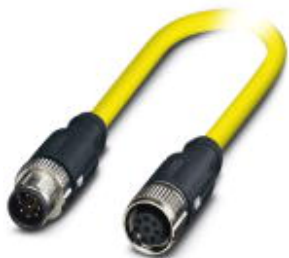
Sensor/actuator cable, 8-position, PVC, yellow, shielded, Plug straight M12 SPEEDCON, coding: A, on Socket straight M12 SPEEDCON, coding: A, cable length: 10 m
