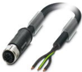
Power cable, 3-position, PVC, black, free cable end, on Socket straight M12, coding: S, cable length: 10 m, for AC current up to 16 A/230 V
